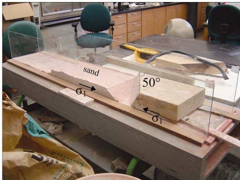
Figure 13. Photograph of pre-deformation sandbox analogue model setup. Sand was pushed against a stationary wood block cut at a 50° angle to \sigma_1 , recreating the stress field of the backlimb of the Miners Mountain uplift.
